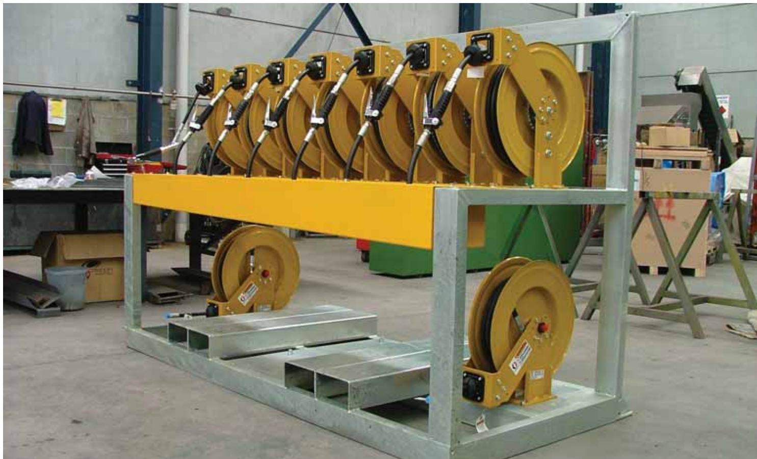
Above: The 504 Diesel Service Bay new hose reel arrangement prior to going underground.
