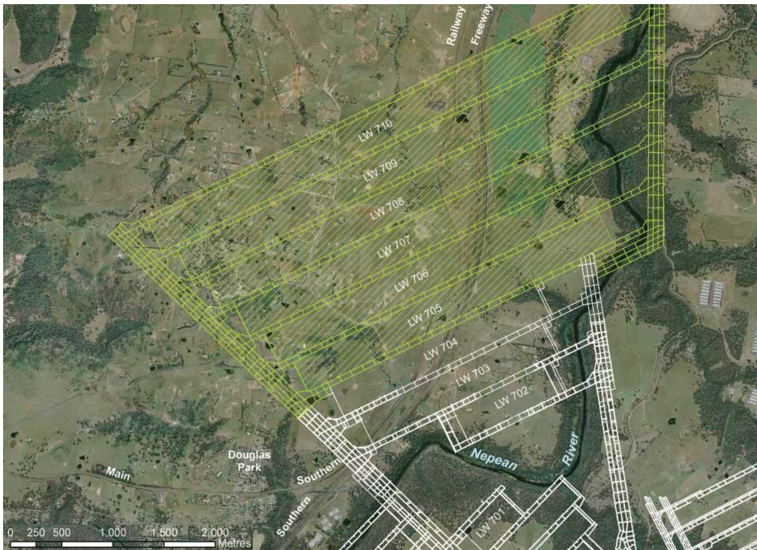
Above: A Subsidence Management Plan has been submitted seeking approval for Longwalls 705 to 710 (Appin Mine).
